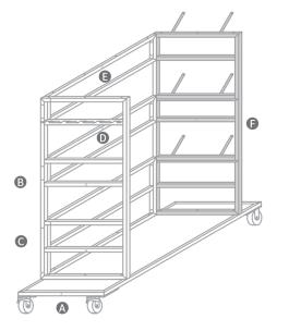
6. Connect the G top plate to the B, E, and F frames and tighten the screws
