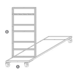
3. Connect the C frame to the B frame and the A base, and tighten the screws
