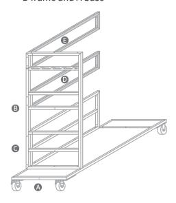
5. Connect the F frame to the C, D, E frames and A base Tighten the screws
