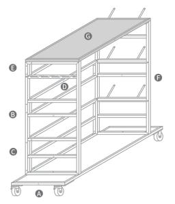
7. Connect the H and | shelves to the B frame and F frame respectively and tighten all the screws.
