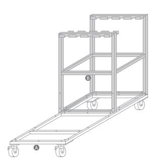
3. Connect the C frame to the B frame and A base respectively.
