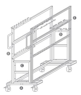
5. Connect the F frame to the B frame and E frame respectively and tighten all the screws.
