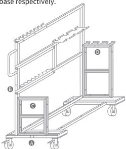
4. Connect the E frame to the C frame, D frame and A base respectively.
