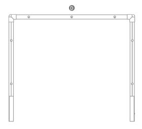
4. Insert the D assembly into the turntable column.
